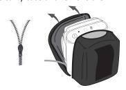
OPEN GREY COVER & INSERT FLUID CONTAINER PACK Insert in the orientation shown. Push firmly until it clicks.
