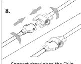
Connect dressing to the Fluid Container Pack. Push connector together and twist to lock.
